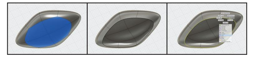
Double click an edge of the hole on quadball(will select entire ring of hole). In the pop-up wheel menu, select "Fill Hole" in the drop down. In the dialog box on the right, change the Fill Hole Mode to "Collapse". Click the check box for "Maintain Crease Edges". Click "Okay" to accept. At the top of the toolbar, click "Finish Form" to exit the sculpting environment.
