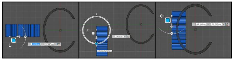
• Change to the top view, use the arrows on the gizmo to position the letters onto the cuff as you desire. Also use the rotation arc to change the angle of the letters to match the cuff curve. Position the letters so they will also intersect cuff.
