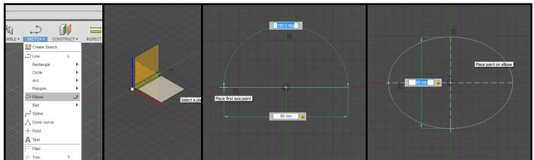
• Add thickness to the cuff. To do this, in the tool bar at the top, click "Sketch ▼ " to expand the menu, click "Offset" (or press "O" on keyboard), and select ellipse. Change the offset value to "3.00mm" outward and press enter/return to accept.
