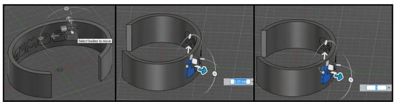
• Use the move tool to offset letters from the cuff "1.00mm". To do this, select the move tool from the menu or press "M" on the keyboard, click the arrow pointing away from the outside of cuff as shown in reference image, and set value to "1.00mm". Continue to position the remaining letters individually.
