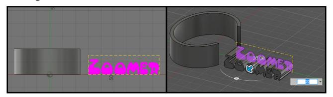
Use the extrude tool to extrude text to "20.00mm".
