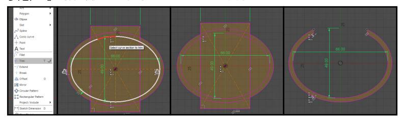
• In the tool bar at the top, click "Sketch ▼ " to expand the menu, and click "Trim" (or press "T" on the keyboard). To trim an unnecessary part of the sketch, hover over the line, the line will turn red if removable, and click to remove. Continue trimming the sketch until it looks similar to the sketch shown above.
