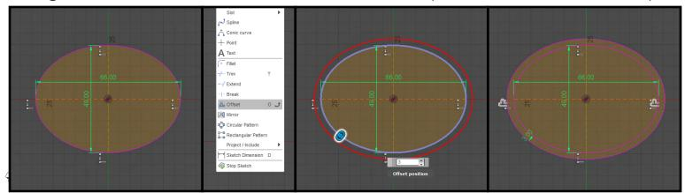
• In the tool bar at the top, click "Sketch " to expand the menu, click "Rectangle ", and click "Center Point Rectangle". Click the center point of origin to place the center point of the rectangle. Set the width value to the "pinch height" and set the height of the rectangle to intersect the outside ellipse as shown.
